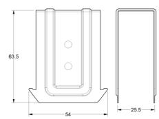
GypFrame® PRIMA Coupling Bracket is used to connect furring channel to main runner.
